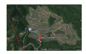
An HV pylon route is 200m to the west (red), but no connection to the solar farm is visible.
